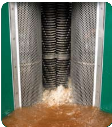
Wastewater entering a Channel Monster grinder.
